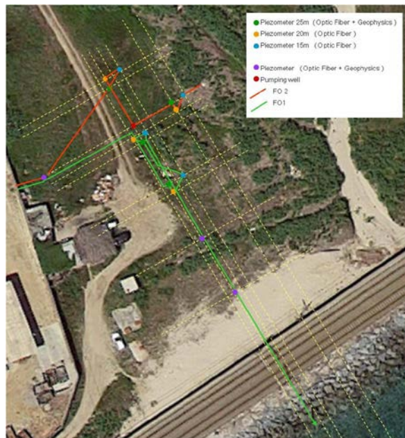
Figure 1. Field site Riera Argenta. Distribution of Fiber Optics cable.
