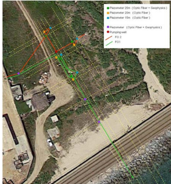
Figure 1. Field site Riera Argentona. Distribution of Fiber Optics cable.
